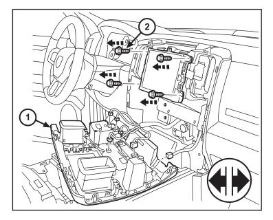
52. Remove radio assembly (1) from dash. Unlock the the 52-way connector (2) at the back of the radio and disconnect.
