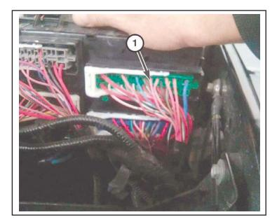
30. Place the strands of the wires overlapping each other inside of the splice clip (1).
