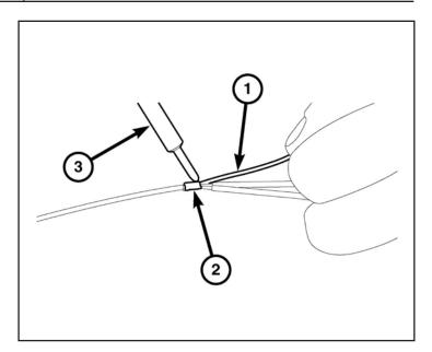
33. Center the heat shrink tubing (2) over the solder joint and heat using a heat gun. Heat the joint until the tubing is tightly sealed and sealant (1) comes out of both ends of the tubing.
