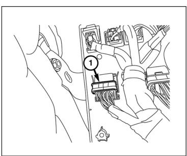
42. Remove the housing (2) to gain access to the terminal blocks (1).
