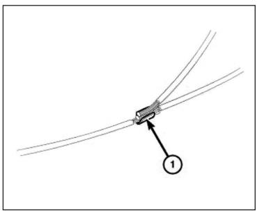
31. Using Mopar® crimping tool (1) or equivalent, crimp the splice clip and wires together.
