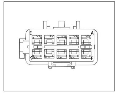
41. Release and remove connector C5 (1) from the Body Control Module (BCM).
