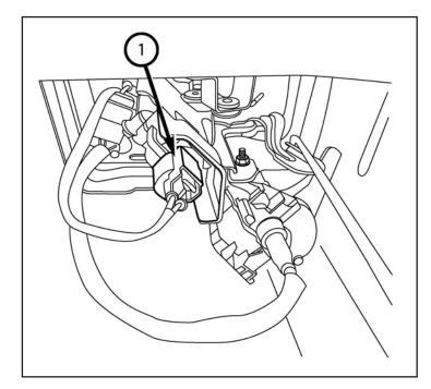
15. Route tailgate jumper harness (D) through the tailgate as shown to the tailgate closeout panel (2).
