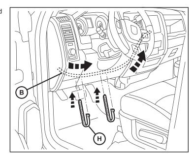
54. Feed the three-prong end of radio harness (B) up into the center stack and out through the radio opening.
