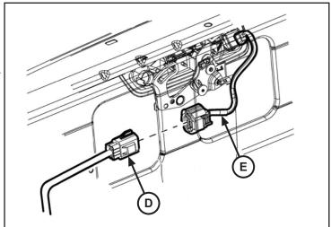
NOTE: Tape back the lock actuator connector if vehicle is not equipped with a lock actuator.
