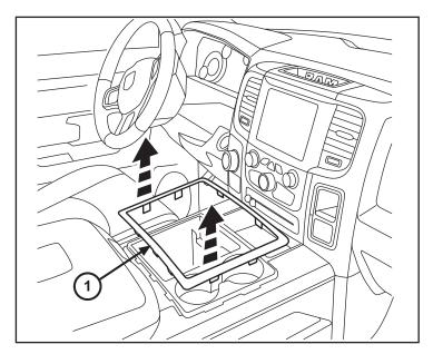
48. Remove fasteners (1) at the front edge of the center console cover panel (2). Remove the cover panel.
