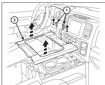
49. Remove fastener (1) from the storage cubby on the right side of the center dash trim panel. Carefully disengage all retainer clips and pry off the trim panel (2).
