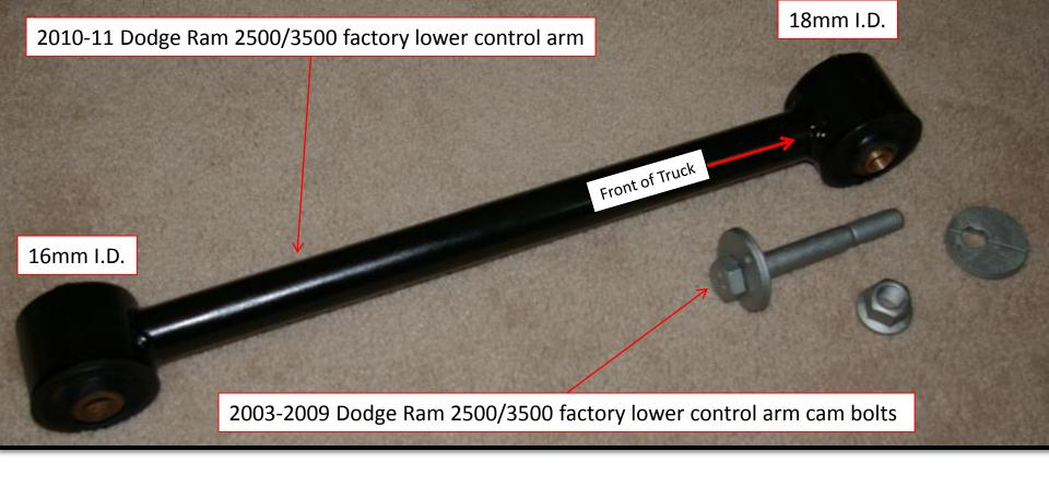
Replacing 2003-2009 stock stamped lower control arm with the Stronger 2010-2011 Tubular steel versions.
