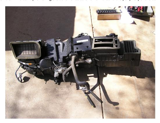
With each door, remove the actuator by removing the two Phillips-head screws and disengaging from the coupler. Take a set of needle nose pliers and pull the coupler straight out of the door axle. Once the coupler is removed, the door falls out. Reinstall in reverse with Heater Treater door and steel coupler, and actuator (don't worry about door position) into/onto the housing.
