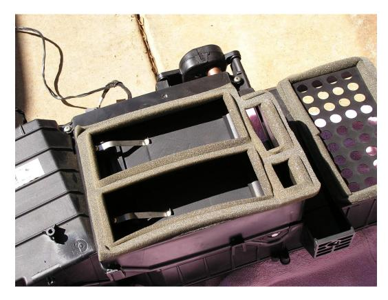
Reassemble HVAC together with Recirculation housing and reinstall back onto firewall and reinstall dash. Be careful to not damage the airbag harnesses near the bottom center of the firewall, which would be located just under the cup holders on automatic transmission trucks. The dash is <u>A LOT</u> heavier than I was expecting and it is very feasible to damage the airbag connections.
