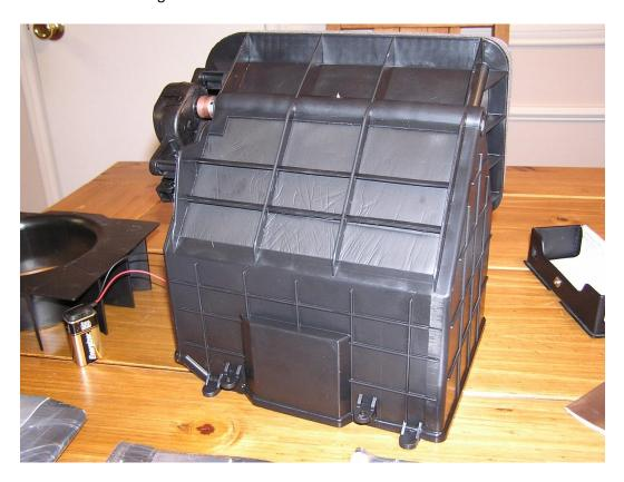
When removing the HVAC box from the firewall, I found it easier to disconnect the heater lines from the engine instead of at the firewall. There isn't much room up underneath the cowl and made the disconnection go more quickly with less skinned knuckles and frustration.
