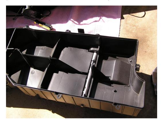
Blend door replaced. You'll notice the arm that connects to another door below the heater coil via a rod and are actuated together. This door is not replaced, but I cannot think of a single incident where that door has broken. It doesn't engage anything; it just rotates on its axle:
