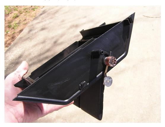
Fin sensor left in place. I have never had the freezing-up issues that others have reported and where the relocation of the sensor was the remedy. I figured, if it ain't broke, don't fix it.
