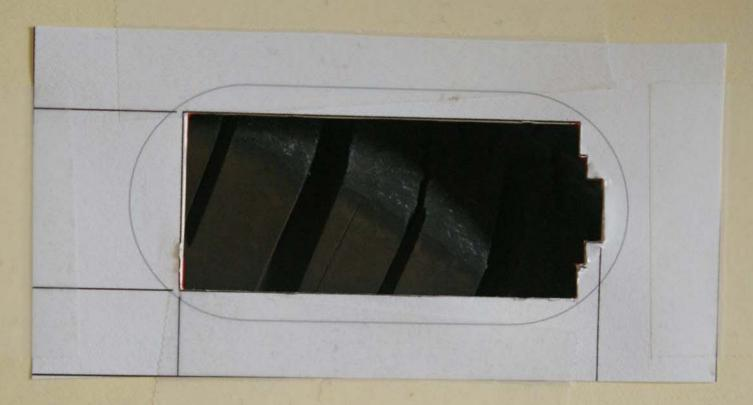
Tape off fender, Locate position based on side marker type
