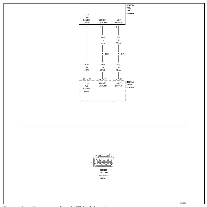
For a complete wiring diagram, refer to the Wiring Information.
