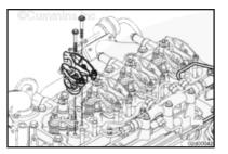
Install the exhaust rocker and adjust the exhaust valve lash. Refer to Procedure 003-008.
