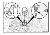
Make sure the injector bore is clean and that only one (1) sealing washer is installed on the injector nozzle.
