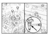
Install the injector hold-down and injector hold-down capscrews, but **do not** tighten. A new high pressure fuel connector **must be used** anytime an injector is replaced.
