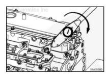
The injector solenoid terminals will yield and may malfunction if too much torque is applied. Do not over tighten.
