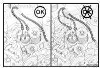
Connect and tighten the solenoid wires.
