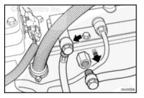
Isolation of the fuel rail pressure relief valve flow from the injector return flow requires the use of the fuel rail pressure relief valve flow tester kit, Part Number 4918295.
