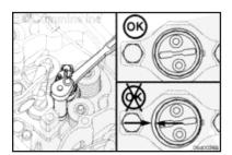
Tighten the injector hold-down capscrews.
