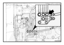
**NOTE:** The fuel return manifold on marine engines is located on the side of the engine block, in front of the ECM.
