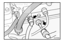
For engines with a quick-disconnect fitting on the fuel rail pressure relief valve, use a female quick-disconnect drain hose and a block-off fitting to isolate the fuel pressure relief valve flow.
