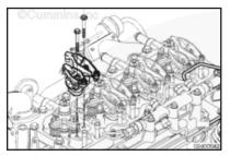
Remove the exhaust rocker lever. Refer to Procedure 003-008.
