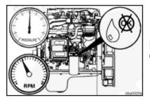
For Marine applications, open fuel supply and return valves. Operate the engine and check for leaks.
