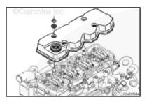
Install the rocker lever cover. Refer to Procedure 003-011.
