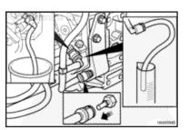
To prevent high pressure fuel pump drain flow from entering the injector return flow, remove the fuel drain line from the high pressure fuel pump.
