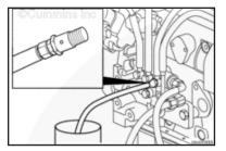
Remove the banjo bolt from the injector drain line at the fuel return manifold.
