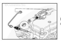
Install the high-pressure fuel line from the fuel rail to the high-pressure connector. Refer to Procedure 006-051.
