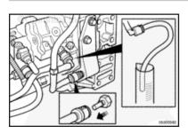
Remove the quick-disconnect fitting on the fuel drain line from the fuel return manifold.
