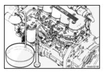
Repeat the leakage flow test with cylinder one blocked off and record the flow rate.
