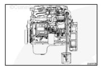
ace the loose end of the fuel pressure gauge adapter tool into a graduated cylinder, Part Number 3823705.
