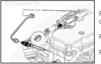
Remove the high-pressure fuel line from the fuel rail and high-pressure connector. Refer to Procedure 006-051.
