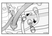
For engines with a banjo fitting on the fuel rail pressure relief valve, use the fuel rail pressure relief valve flow tester kit, Part Number 4918295.
