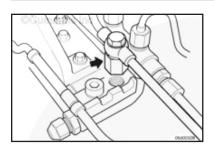
Measurement of injector return flow requires the use of a fuel system leak tester, Part Number 4918354. The fuel system leak tester contains Part Numbers: 4918297, 4918433, and 4918434.
