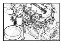
Follow the fuel drain line from the back of the cylinder head to the fuel return manifold. Remove the banjo bolt from the fuel injector drain line at the fuel return manifold. Install the fuel drain hose, Part Number 3164618, in place of the banjo bolt.
