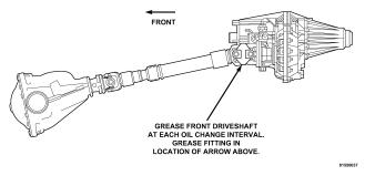
Front Driveshaft Grease Fitting
