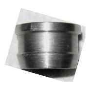
Top Diameter = 36.8 mm (1.45 in) Thickness of top flange is 5 mm (0.20 in)
