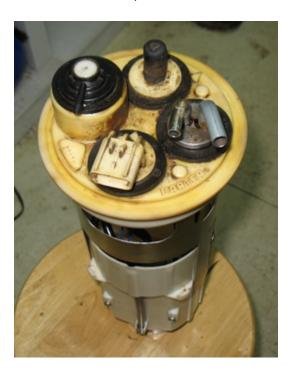
The final installation of the fuel sending module into the tank looked like this.
