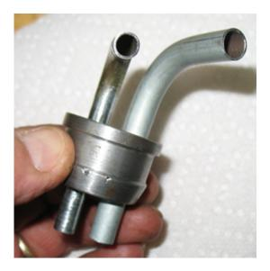
I then had to modify the fuel and return line connection inside the fuel sending module, cutting out the rotten stuff, shortening some lines and fitting some fuel hose to connect to the bottom of the plug. The mods inside looked like this:
