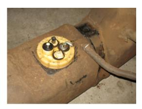
After that, it was almost a full day's work for an old retired guy like me getting the tank back up and into place and connecting new fuel and return line hose. I started the truck and let it run for about 25 minutes to make sure that all was OK. Anyway, it seems so but it has not left the garage yet, so I'm not sure how it will perform on the highway. I'm hoping all will be well.
