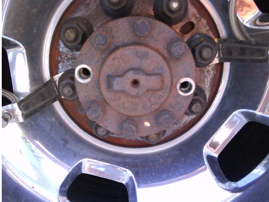
PHOTO 1: Axle shaft Flange Bolts Removed
