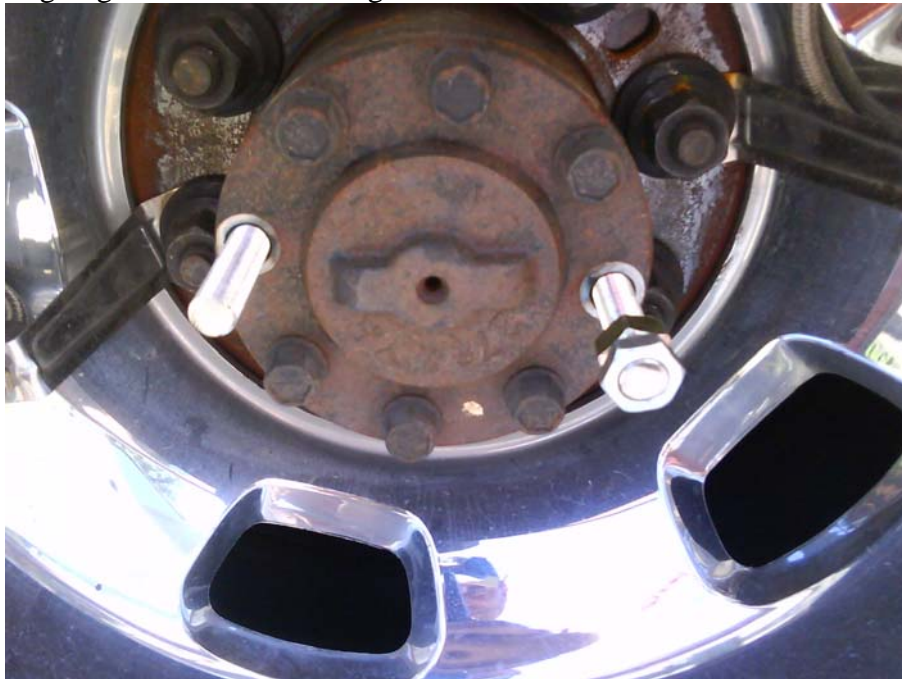
Photo 2: Installing Axle Studs
