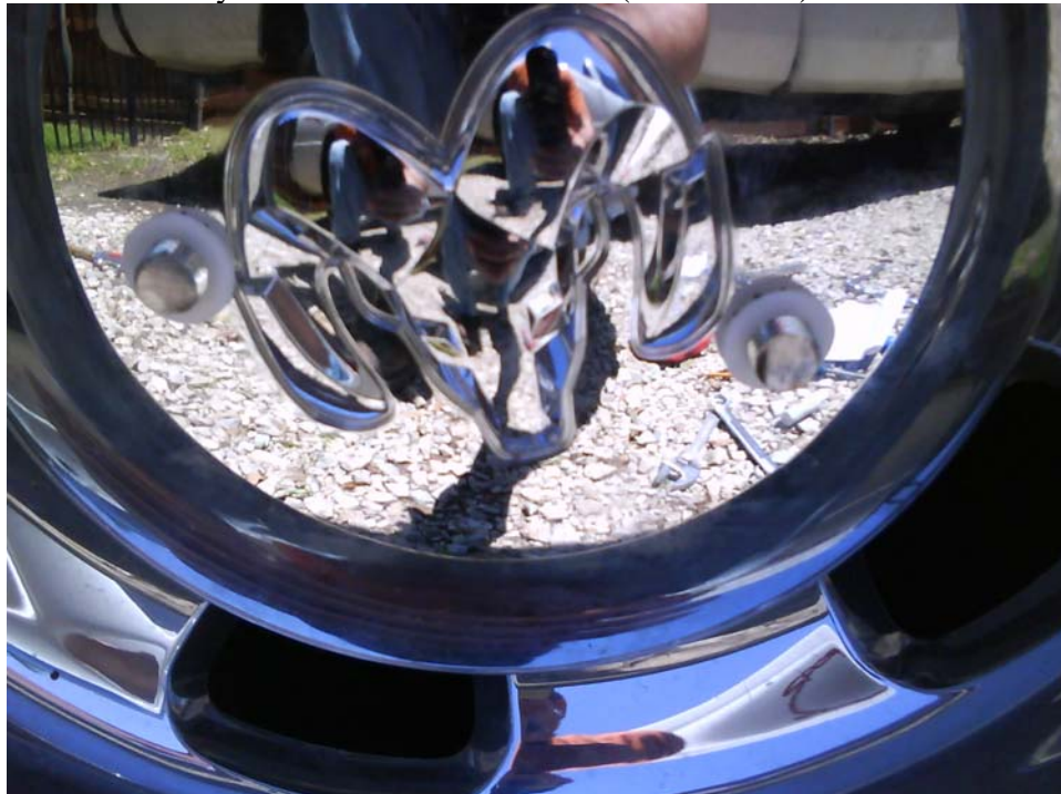
Photo 6: Nylon Washers Installed
